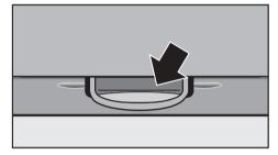
The lower part of the inner door has a drip tray. Clean the drip tray.
